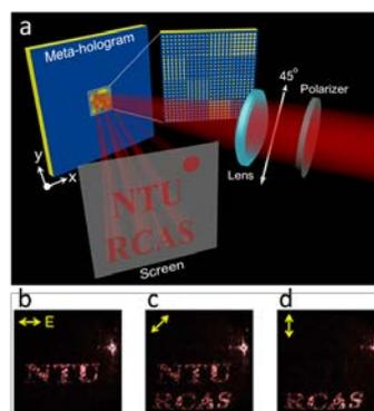
Figure 1. (a) The functionality of our designed meta-hologram under linearly-polarized illumination. Reconstructed images of meta-hologram for case of (b) x-polarized, (c)  $45^\circ$ -polarized, and (d) y-polarized incidence by a 780-nm laser.
