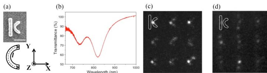
Fig.1 (a) SEM micrograph of hybrid gold nanostructure that consists of curvilinear and straight nanorods with 10 nm gap. The scale bar is 100 nm. The figure shows the layout of curvilinear nanorod and polarization. (b) Transmittance spectrum under the linearly polarized illumination of x-direction. PEEM images of hybrid nanostructures excited using NIR femtosecond laser under the x-direction polarized at the center wavelength of (c) 740 nm and (d) 770 nm.
