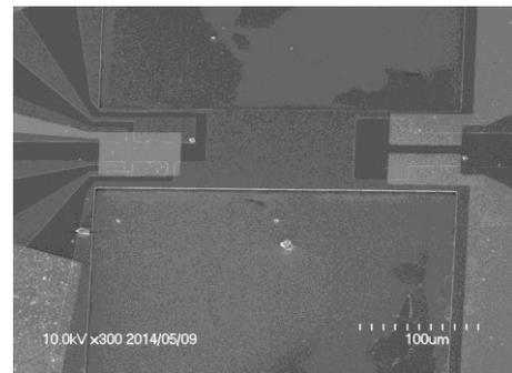
Fig. 1 SEM image of a fabricated doubly clamped beam structure
