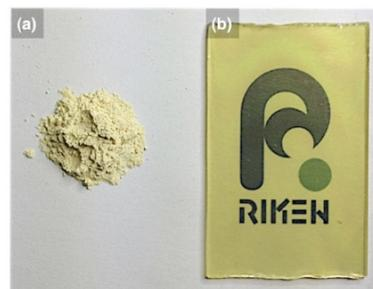
Figure 2. Photograph of (a) powdery graphitic carbon nitride (GCN) and (b) GCN thin film prepared by vapor-deposition polymerization on a glass substrate.
