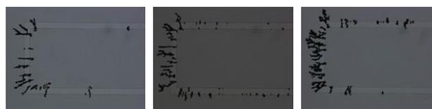
Fig. 2 Dielectrophoretic trapping of Ag nanoparticles
