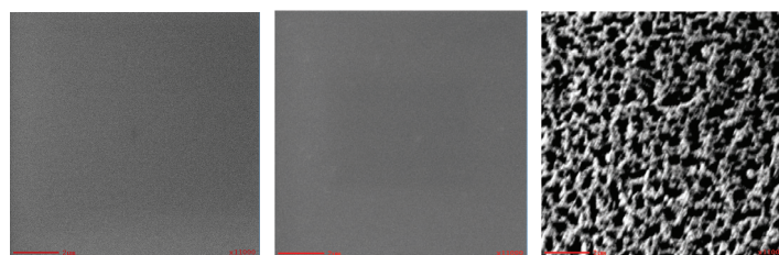
Fig.2 SEM images of SiO_2 (left panel), SiON formed at 10^2 Pa (middle panel), and SiON formed at 5 \times 10^{-1} Pa (right panel). The field of view of each image is 10.8 \times 10.8 \mu m^2 .
