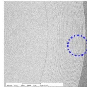
Fig. 2 Fabricated SZFZP for  $\lambda = 13.5$  nm.
