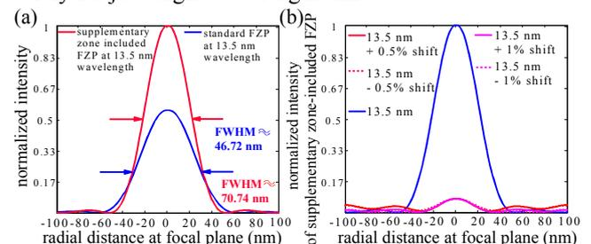
Fig. 3 Lateral profile of the simulated EUV light focus. (a) Comparisons between the standard FZP and the SZFZP. (b) Focuses of the SZFZP when EUV light contains 2% bandwidth.
