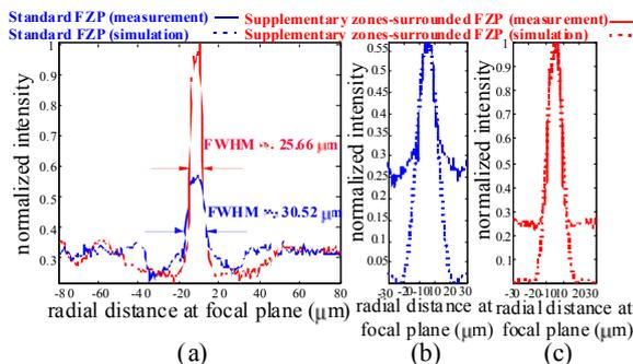
Fig. 1 Lateral profile of the red light focus, where (a) stands for the measurements, (b) stands for the simulated and measured profiles for the standard FZP, and (c) stands for the simulated and measured profiles for the SZFZP.
