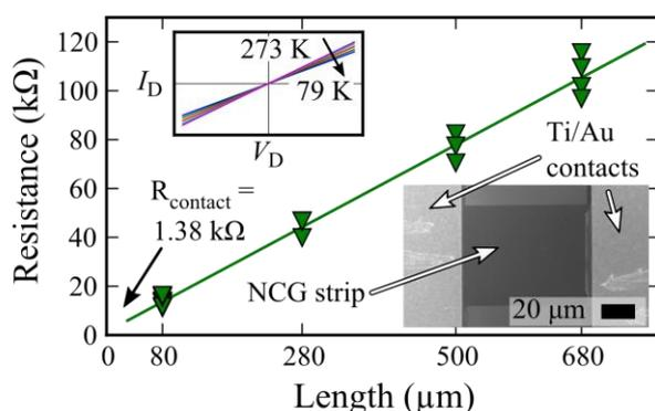
**Fig. 1.** Room temperature resistance of 60  $\mu\text{m}$  wide NCG strips with various lengths. A 80  $\mu\text{m}$  long device is shown lower right inset. The  $I_D/V_D$  results used for linear fitting are shown in upper left inset.
