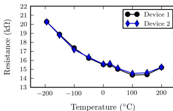
**Fig. 2.** Resistance of 60  $\mu\text{m}$  wide and 80  $\mu\text{m}$  long NCG devices for different temperatures.
