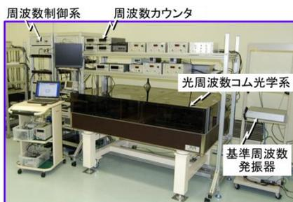
Fig.1 Our laser frequency calibration system
