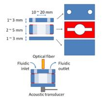
Fig. 1 Schematic view of the proposed fabrication process based on patterning of acrylic plates (in blue) with CO2 laser cutting tool and bonding with double-side tapes (in red).
