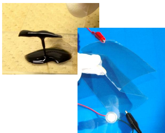
Fig.2 SWNT ink and resulting transparent conductive film prepared on PEN.
