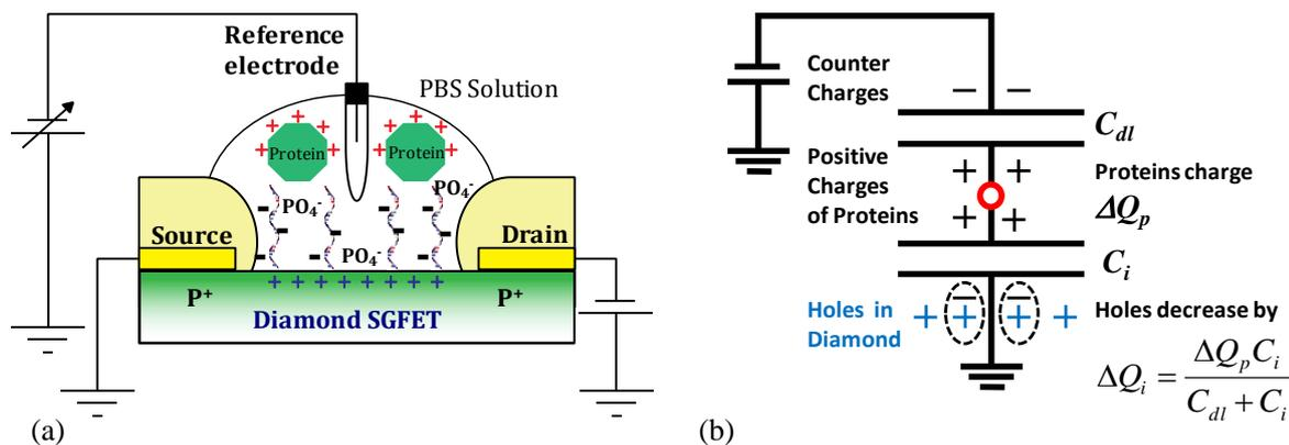
Fig.1 (a) aptamer immobilized diamond SGFET for protein detection. (b) equivalent circuit for charge change  $\Delta Q_p$  between an electric double layer capacitor  $C_{dl}$  and a capacitor on solid side  $C_i$ . [4-7].
