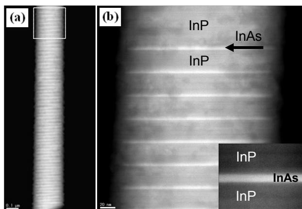
Fig. 1. HAADF-TEM images of (a) a multi-stacked InP/InAs NW with 60 InAs layers (b) the area indicated the dotted line in (a). The scale bar in (a) denotes 100 nm. The scale bar in (b) denotes 20 nm.
