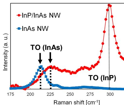
Fig. 2. Raman spectra of a multi-stacked InP/InAs NW and a pure InAs NW. TO phonon peaks from the InAs and InP segments of the two NWs are indicated.
