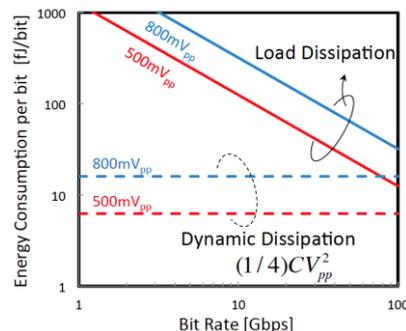
Fig. 3: Prospects for energy power consumption per bit as a function of bit rates. Two factors of the dissipation in 50 ohm load resistor and the dynamic dissipation in capacitive charging and discharging are considered.
