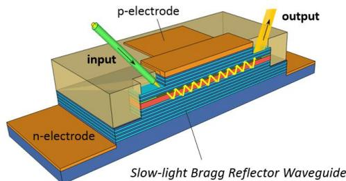
Fig. 1: A schematic cross-section view of the slow-light Bragg reflector waveguide modulator.
