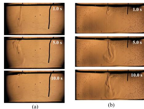
Fig. 2. Schlieren images of liquid anode discharge at 10 mA. (a) normal condition, (b) with sheet to prevent the contact between gas flow and liquid surface.
