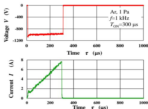
Fig. 2. Discharge V-I characteristics with SMC.
