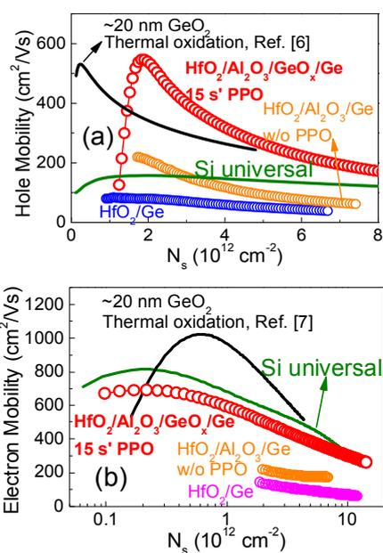
**Fig. 4.** The hole (a) and electron (b) mobility of Ge p- and n-MOSFETs with  $\text{HfO}_2/\text{Al}_2\text{O}_3/\text{GeO}_x/\text{Ge}$  gate stacks.
