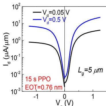
**Fig. 3.** The  $I_d$ - $V_d$  characteristics of Ge p- and n-MOSFETs with  $\text{HfO}_2/\text{Al}_2\text{O}_3/\text{GeO}_x/\text{Ge}$  gate stacks.
