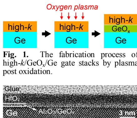
**Fig. 1.** The fabrication process of high- $k/\text{GeO}_x/\text{Ge}$  gate stacks by plasma post oxidation.
