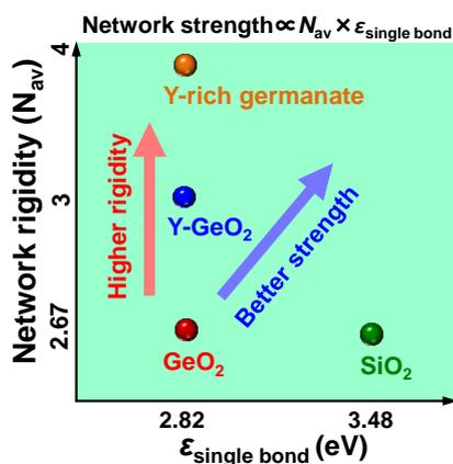
**Fig. 1** Schematic on the definition of network strength and rigidity. GeO<sub>2</sub>, 10% Y-GeO<sub>2</sub> and Y-rich germanate are examples with different  $N_{\text{av}}$  value and network strength.
