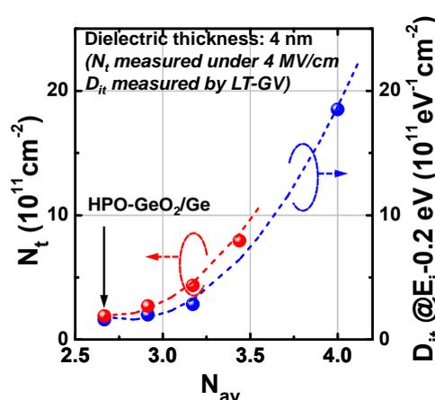
**Fig. 2**  $N_{\text{t}}$  for electron and  $D_{\text{it}}$  near mid gap in dielectric/Ge gate stack as a function of  $N_{\text{av}}$ . Note that the  $N_{\text{t}}$  is estimated from the  $V_{\text{FB}}$  shift by:
