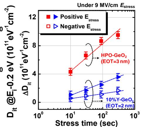
**Fig. 3**  $D_{\text{it}}$  increase in HPO-GeO<sub>2</sub> and 10% Y-GeO<sub>2</sub>/Ge stacks as a function of time under positive or negative 9 MV/cm  $E_{\text{stress}}$ . Note that HPO-GeO<sub>2</sub> break down under 9 MV/cm negative  $E_{\text{stress}}$
