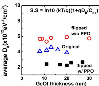
Fig.4: Thickness dependence of average  $D_{it}$  value of different back interface from S.S factors
