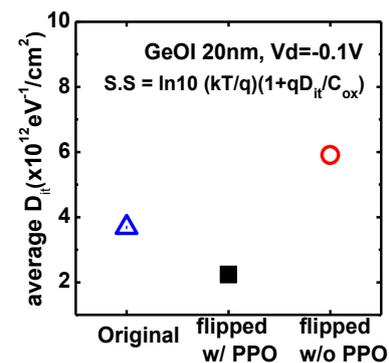
Fig.2: Average value of  $D_{it}$  estimated from the S.S factors of 20nm GeOI with different back interface
