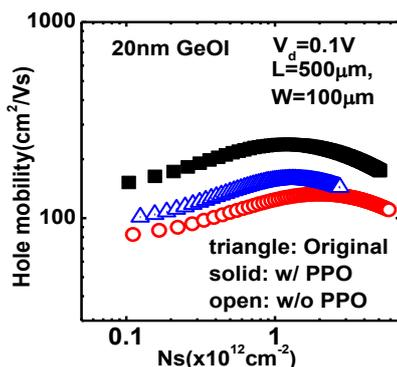
Fig.3: Effective hole mobility of 20nm GeOI with different back interface
