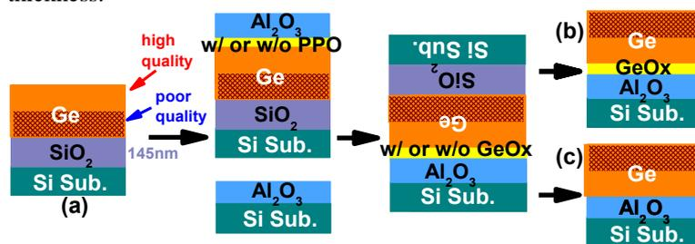
Fig.1: Process flow of flipped GeOI fabrication and the GeOI with different back interface (a) original GeOI (b) flipped GeOI with PPO (c) flipped GeOI w/o PPO
