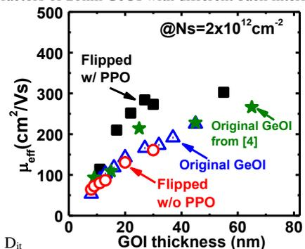
Fig.5: Thickness dependence of hole mobility
