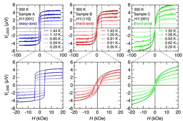
Figure 1: External-magnetic-field dependence of longitudinal spin-Seebeck signal ( $V_{LSSE}$ - $H$ ) measured at 300 K in Pt/CFO bilayers grown on MAO(110) (blue and red) and MgO(001) (green) substrates.
