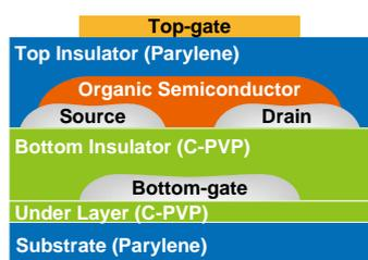
**Fig. 1.** The device structure of the fabricated DG-OTFT
