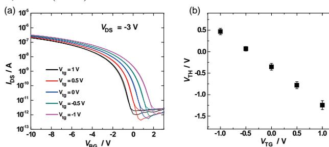
**Fig. 2.** (a) The transfer characteristics of the DG-OTFT. (b) The relationship of the  $V_{TH}$  and  $V_{TG}$ .
