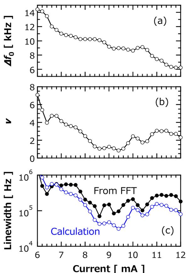
Figs. 1 Current dependence of (a)  $\Delta f_0$  and (a)  $v$ , and (c) linewidth.
