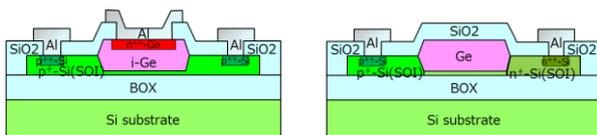
Fig.1 Cross Sections of Waveguide Butt-Joint Ge-PIN-PDs
