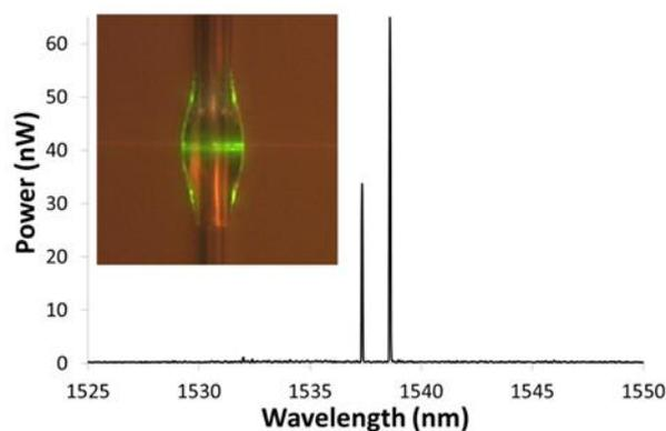
Fig. 1. The lasing spectrum from an Er:Yb doped glass microcavity formed on the outer surface of a microcapillary with a diameter of 70  $\mu\text{m}$ . Inset: image of the microlaser.
