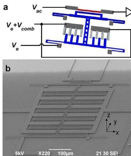
Figure 1. (a) A simplified schematic of the beam, movable electrode and comb actuator. (b) Scanning electron micrograph of the device.
