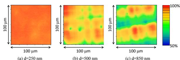
Fig. 2. PL maps of template after annealing at 610 °C for various template thicknesses.
