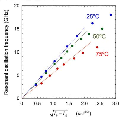
Fig. 3. Modulation efficiency of membrane DFB laser.
