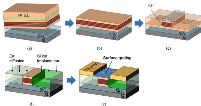
Fig. 1. Fabrication procedure for membrane laser.
