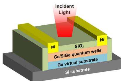
Figure 1. Schematic plot of the Ge/SiGe QW photoconductors.
