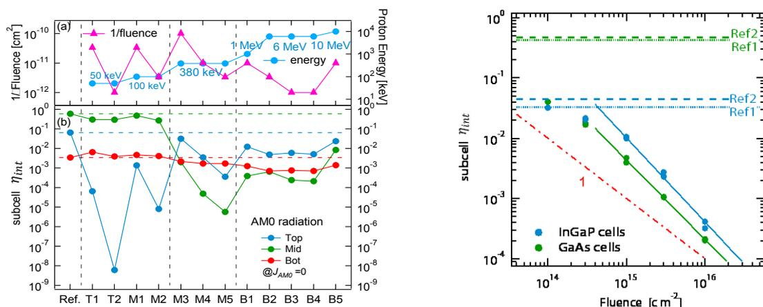
Fig. 1 (a) Plot of incident proton energy and fluence of reference sample and 12 proton-irradiated 3-junction samples (b) Plot of evaluated top-, middle-, bottom-cell  $\eta_{int}$  at the open-circuit condition under AM0.
