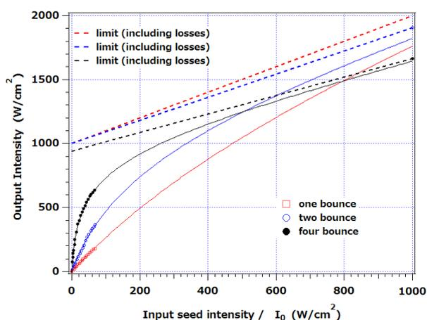
**Fig. 1.** The amplifier output- versus the input seed beam intensity dependence for one, two and four bounce amplification cases including linear losses. The excitation beam power and spot diameter were  $\sim 405 \text{ W}$  and  $\sim 4 \text{ mm}$  ( $3.23 \text{ kW/cm}^2$ ), respectively. The fitting curves were obtained by using an analytical approximation based on Frantz-Nodvik equation [2] including experimentally determined linear losses.
