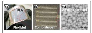
Figure 1. Microprinting of Ag nanoparticle on PLA film.
