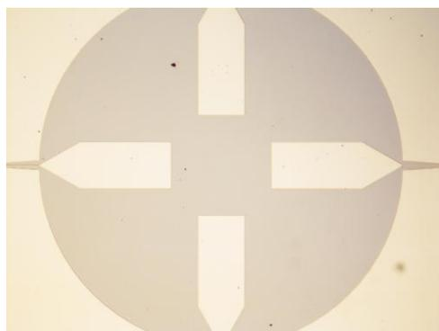
Fig.1 Planar OMT of horn coupled MKID
