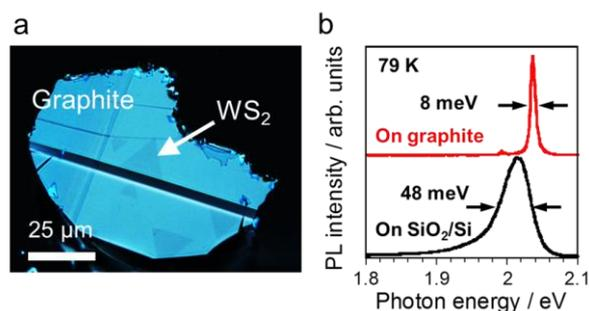
Figure 1. (a) Optical image of WS<sub>2</sub> crystals on graphite. (b) Photoluminescence spectra of WS<sub>2</sub> grown on graphite (red) and SiO<sub>2</sub>/Si (black) substrate at 79 K.
