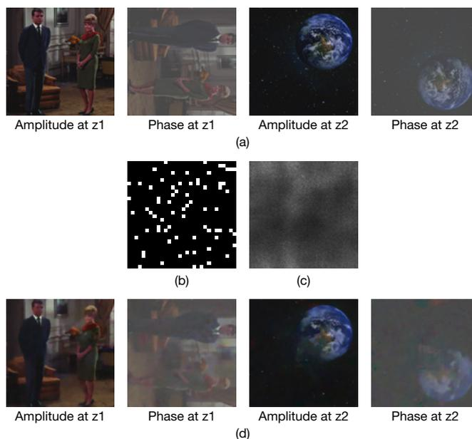
Fig. 2. Simulation results. (a) Object, (b) magnified image of the coded aperture, (c) captured image, (d) reconstruction.
