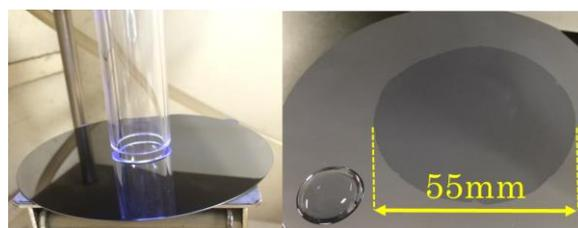
Fig.2 Effective irradiation range of atmospheric pressure plasma generator (55mm)
