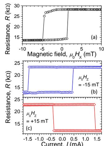
Fig. 2:  $R$ - $H_x$  (a) and  $R$ - $I$  loops (b,c).
