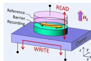
Fig. 1: Structure of proposed device.
