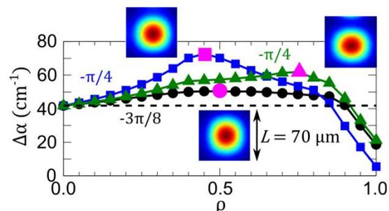
**Fig. 2** Threshold gain difference  $\Delta\alpha$  versus reflectivity  $\rho$  for uniform left boundary (black), uniform top and left boundaries (blue), and non-uniform top and left boundaries (green) when  $\phi$  is fixed to the indicated value. The dashed line is  $\Delta\alpha$  when  $\rho = 0$  everywhere. The insets are field intensity profiles at the highlighted points.
