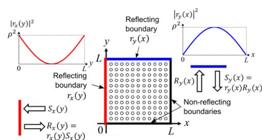
**Fig. 1** Exemplary schematic of reflection at the left ( $x=0$ ) and top ( $y=L$ ) boundaries of a square-lattice PC of side length  $L$ .  $S_x(y)$  and  $R_y(x)$  are outgoing basic waves.  $R_x(y)$  and  $S_y(x)$  are incoming basic waves. All basic waves are spatially dependent.
