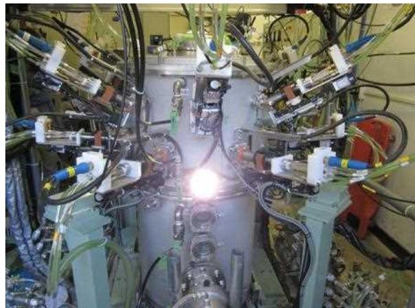
Fig. 2 Multi-phase AC arc for nanoparticle synthesis
