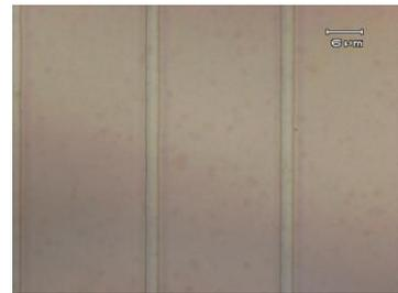
Fig.2 Optical microscope photograph of top view of LN ridge waveguides.
