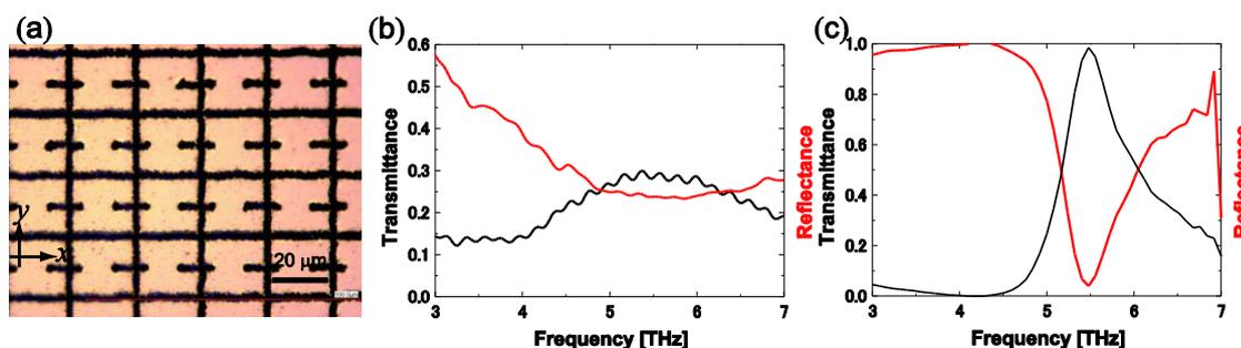
Fig. 1 (a) The microscope image of the metamaterial structure. Measured (b) and FDTD simulated (c) transmittance (black curve) and reflectance (red curve) spectra for the metamaterial, respectively.
