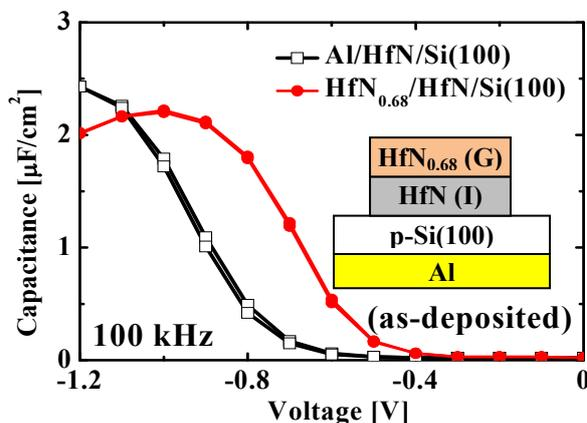
Fig. 2. C-V characteristics (100 kHz) of as-deposited HfN/p-Si(100) MIS-diode with Al and HfN gate electrode.
