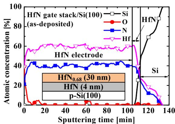
Fig. 1. Depth profile of *in-situ* HfN gate stack structure formed by ECR plasma sputtering.
