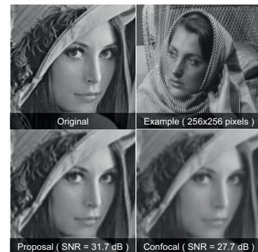
Fig. 2 (a) Original sample image, (b) example image, (c) reconstructed image and (d) confocal image.
