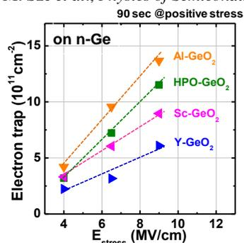
**Fig. 1** Electron trap density generated in HPO-GeO<sub>2</sub> and M-GeO<sub>2</sub>/Ge stacks as a function of  $E_{stress}$  for 90 sec.
