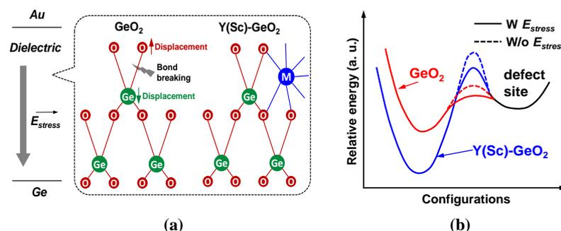
**Fig. 2(a)** Schematic of Y(Sc)-GeO<sub>2</sub> MRN structure and its impact on the ion displacement. **(b)** Schematic of energy diagram for the dielectric degradation by  $E_{stress}$  or by thermal decomposition (GeO desorption).
