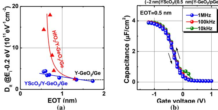
**Fig. 2(a)**  $D_{it}$  @  $E_t = 0.2 \text{ eV}$  as a function of EOT in  $\text{YScO}_3/\text{Y-GeO}_2/\text{Ge}$  and  $\text{HfO}_2/\text{Y-GeO}_2/\text{Ge}$  stacks. **(b)** Bidirectional  $C-V$  curves of a  $(2 \text{ nm})\text{YScO}_3/(0.5 \text{ nm})\text{Y-GeO}_2/\text{Ge}$  stack measured at RT.
