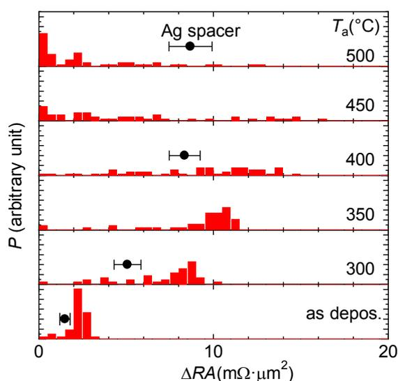
Fig. 1: Distribution of  $\Delta RA$  of the CPP-GMR devices with CuZn spacer for each annealing temperature  $T_a$ . The black dots indicate the average values of  $\Delta RA$  for the devices using Ag spacer [3].
