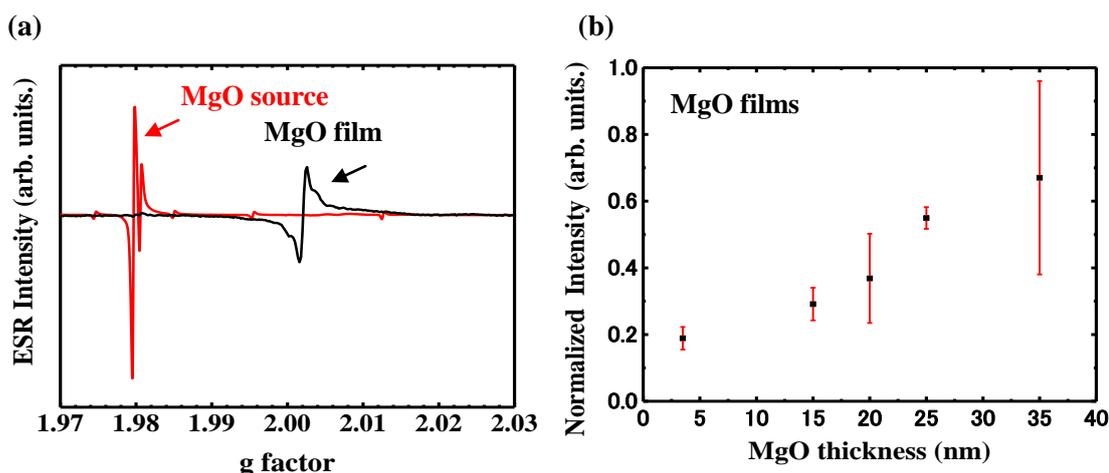
FIG .1 (a) ESR signals of MgO source (red) and MgO deposited film(35nm) (black)
