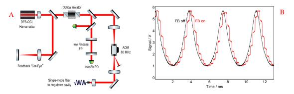
We are pursuing a simpler approach, similar to the one detailed in [3] and shown in Figure A. Our first experimental results demonstrate the effect of feedback on the wavelength tuning behavior of the laser as well as first indications of linewidth narrowing. Measurements were carried out both with a low finesse FPI (Figure B) as well as by monitoring the output of the high finesse cavity used for ring-down spectroscopy.
