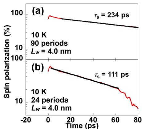
Fig.2 Time evolutions of spin polarization of (a) 90-period-SL sample and (b) 24-period-SL sample at 10 K for excitation power of 110 mW.
