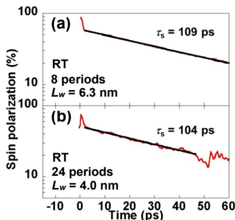
Fig.1 Time evolutions of spin polarization of (a) 8-period-SL sample and (b) 24-period-SL sample at RT for excitation power of 110 mW.
