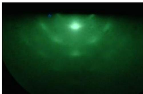
**Figure 1** RHEED pattern of the ultrathin MgB<sub>2</sub> film (10 nm) on a CaF<sub>2</sub> buffer layer.
