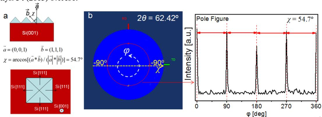
Fig. 1. (a) Schematic diagram of textured Si(001) substrate with (111) faces. (b) X-ray pole figure image with  $2\theta = 62.42^\circ$
