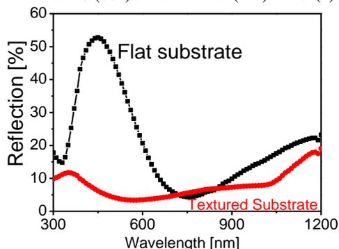
Fig. 2. Reflectance spectrum of undoped-BaSi<sub>2</sub> on flat substrate and textured substrate
