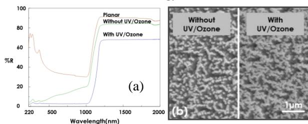
Fig. 1(a) Reflectance spectra from 220 nm to 2000 nm
