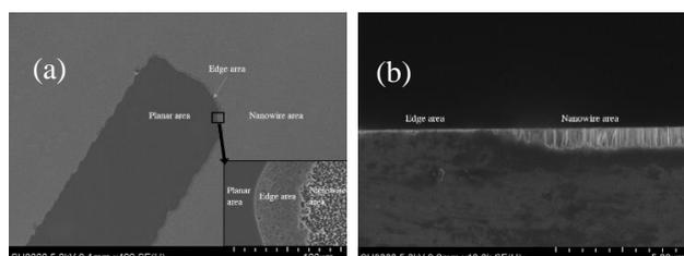
Fig. 2 (a) Top and (b) cross-section view of SEM image of selectively etched silicon substrate.
